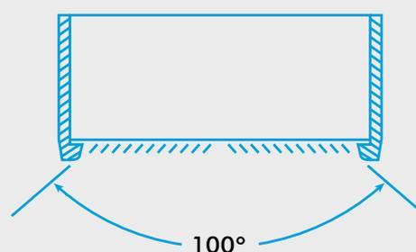
AIR IS BLOWN UP TO 50° IN THE DOWNWARD DIRECTION
