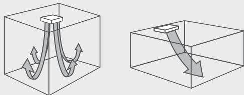
Note: When units are installed on high ceilings, depending on the model, various restrictions concerning maximum height, air discharge direction, and choice of options may apply.
