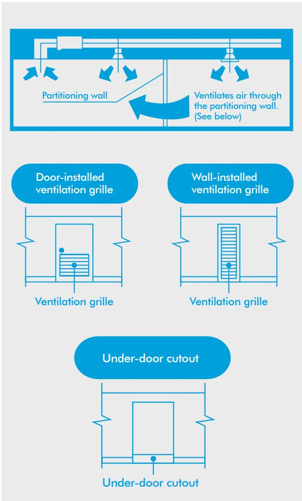
Note: The under-door cutout method should be used only when there is a small volume of airflow.
