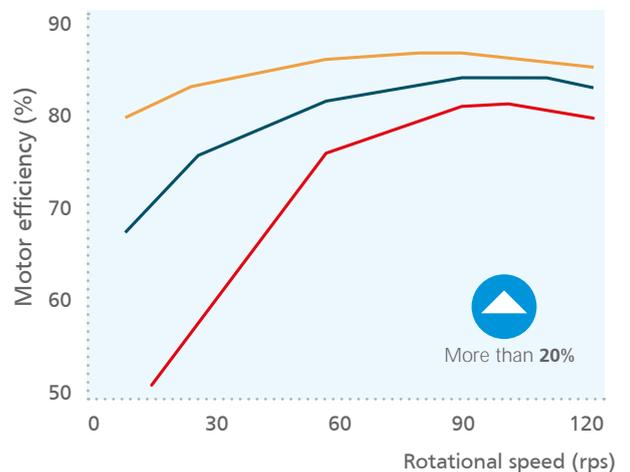
Legend: Reluctance DC motor (orange line), Conventional DC motor (dark blue line), AC motor (red line)
