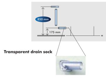
Hanging height adjustment Because the configuration of the hanger bracket changed, the dimensions from the ceiling to the hanger bracket also change during height adjustment for indoor unit.
