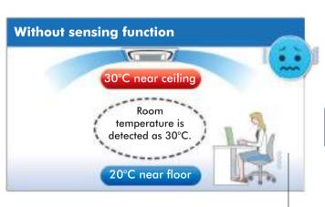
Area around feet gets too cold because the air conditioner continues until the temperature near the ceiling reaches the set temperature.
