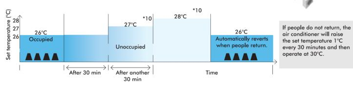
Shift temperature and time can be selected from 0.5 to 4°C in 0.5°C increments and 15, 30, 45, 60, 90 or 120 minutes respectively with remote controller.
