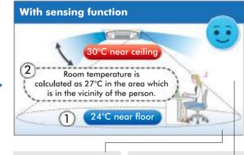
The floor temperature, which is lower than near the ceiling, is detected.
